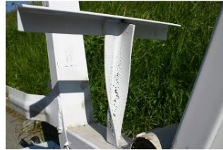
Intentionally twisted (by 90°) steel (equal angle steel) showing permanent deformation. De Sunspandier en Wikimedia Commons. Licencia CC-BY-SA.
