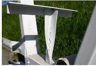
Intentionally twisted (by 90°) steel (equal angle steel) showing permanent deformation. De Sunspearcler en Wikimedia Commons. Licencia CC-BY-SA.
