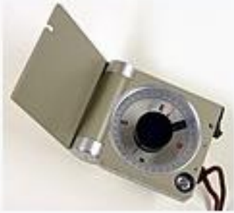
Breithaupt geological compass COCLA with damping of the oscillations of the magnetic needle
